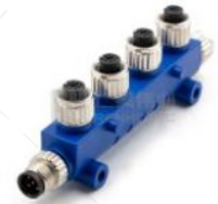
NMEA 2000 CONNECTORS NMEA 2000 4 Way Tee Connector
