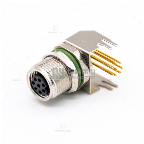
M8 Female Right Angle Receptacle Through Hole Mount with Metal Bracket
