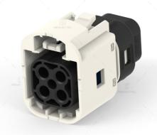
Wire-to-Board Sealable 180° Cable Exit 4 Position B Code Housing for Female Terminals 5 mm (.2 in) Centerline Crimp Data Connectivity Housings
